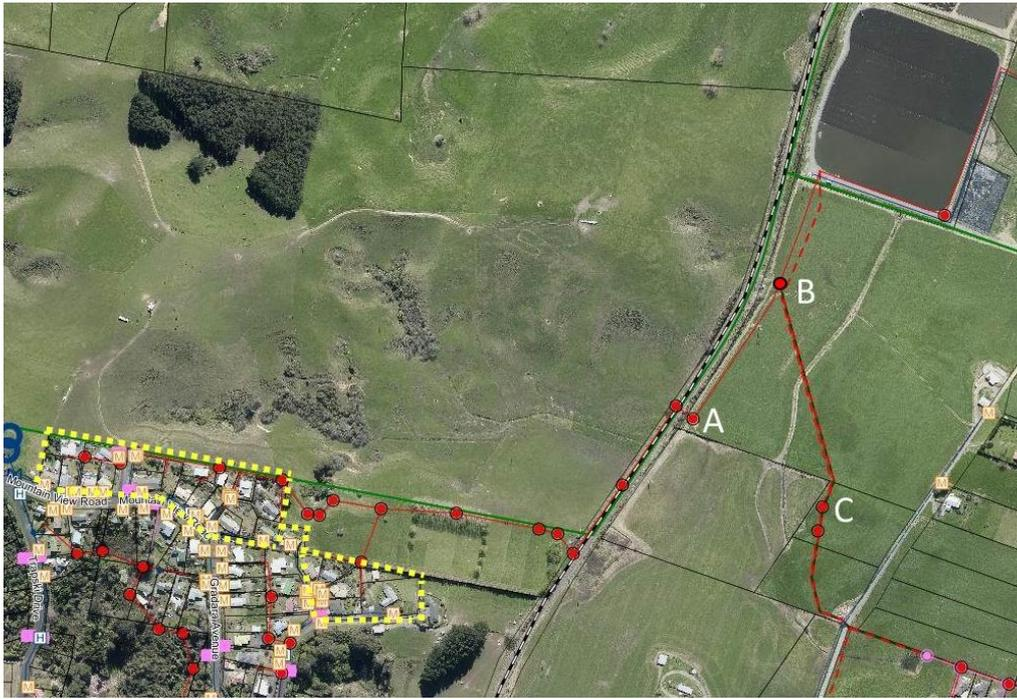
Of the two factors believed to be contributing to the problem – low flows and lack of gradient – only the latter can practically be resolved. It has been previously proposed that an attempt should be made to address the issue by re-laying the pipes between A and B to ensure that the gradient between these two points was uniform, without any ‘sags’ where solids might accumulate. A cost in the order of \$20,000 + GST was estimated for such work.
