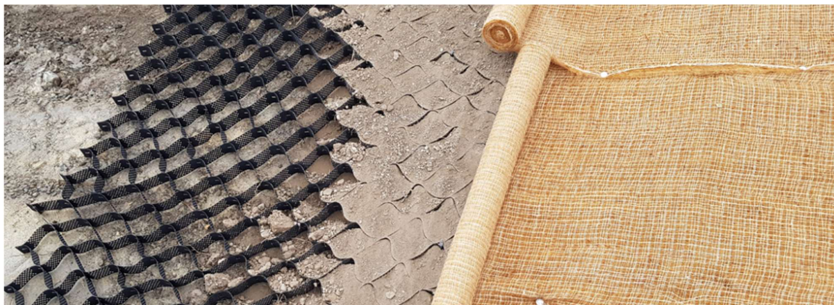
Figure 2.6: Example of Geoweb® with coir matting (Source: www.geofabrics.co.nz )
