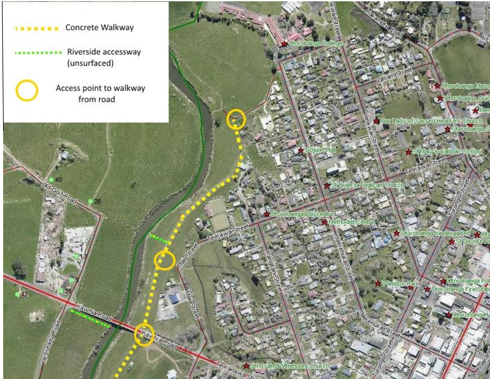
Walkway Section 3: Kawhia Road to Waipa Esplanade (600 metres approximately)
